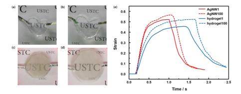
Fig. 2. DEAs fabricated from hydrogel and AgNW compliant electrodes. The initial (a) and activated (b) state of actuators based on heart-like PVA hydrogel. The initial (c) and activated (d) state of actuators based on circular
