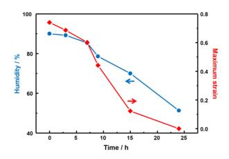
Fig. 4. The influence of moisture content on the electroactivity of hydrogel electrodes.
