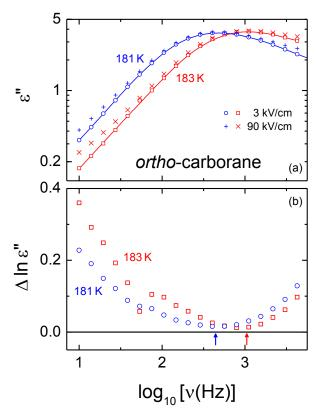
FIG. S1. (a) Dielectric loss spectra of *ortho*-carborane in the plastic-crystalline state for two temperatures, measured at low and high field. The lines are shown to guide the eyes. (b) Difference of the logarithms of the high- and low-field spectra. The arrows indicate the loss-peak positions.
