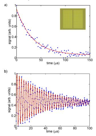
Fig. 5. (color online) (a) Energy relaxation time  $T_1$  of Qubit A (Si substrate) mounted in a Sn-plated copper cavity. Fit to exponential decay corresponds to  $T_1 = 33 \ \mu$ s. The inset shows an optical micrograph of the qubit. (b) Coherence time measurement (Ramsey fringes) for the same qubit/cavity corresponding to  $T_2^*$  of 41  $\mu$ s (based on Fig. 3 in Ref. [15]).
