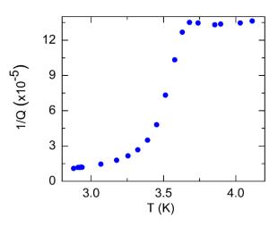
Fig. 4. (color online) Temperature dependence of total loss for an empty Snplated copper cavity measured across the Sn superconducting transition temperature.
