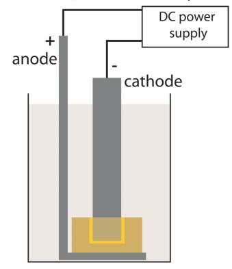
Fig. 2. (color online) Schematic design of the electropolishing setup; the cavity is shown in cross-section. As described in the text, it is essential for the anode to cover the entire back area of the half-cavity.
