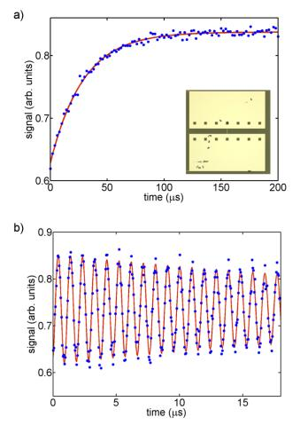
Fig 6. (color online) (a) Energy relaxation measurement of Qubit B (sapphire substrate) mounted in a Sn-plated copper cavity. The inset shows an optical micrograph of the measured qubit. (b) Ramsey fringe measurement for the same qubit/cavity.
