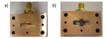
Fig. 1. (color online) (a) OFHC Cu half-cavity that has been electropolished. (b) Half-cavity with the walls electroplated with Sn; a transmon qubit fabricated on a Si substrate has been placed in the chip recess. The SMA connectors are threaded in for different external coupling levels between (a) and (b). The outer dimensions of the OFHC Cu block in which the cavity is machined are  $3.8 \times 2.3$  cm<sup>2</sup> for the open face as pictured above with a height of 1.4 cm.
