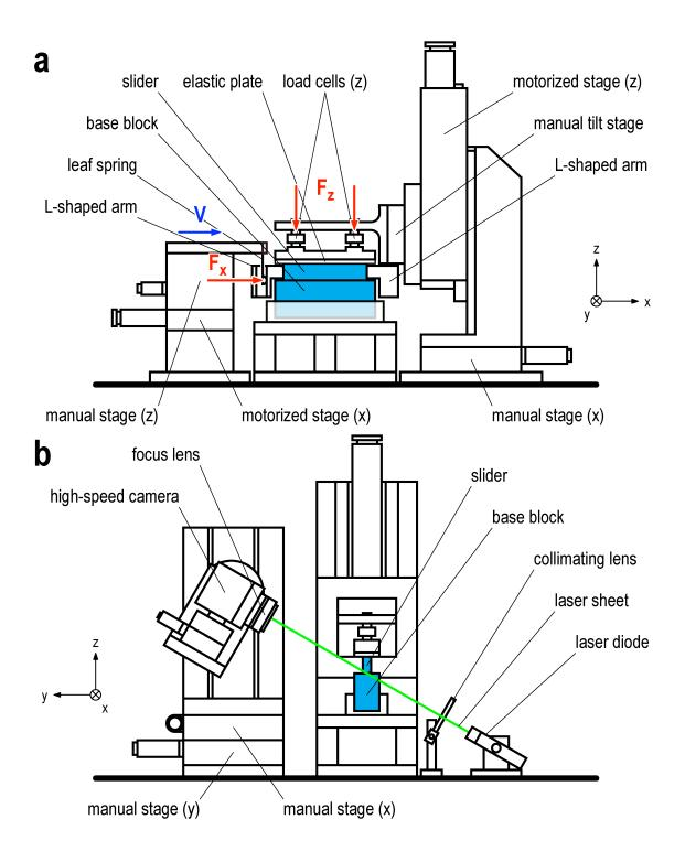
Supplementary Fig. 1: Schematic of the experimental apparatus: (a) front view and (b) side view.
