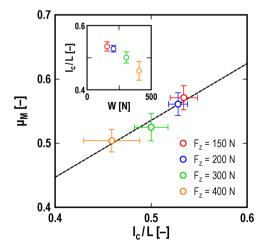
Figure 4 | Macroscopic static friction coefficient  $\mu_M$  vs. critical precursor length  $I_c$ . The dependence of the macroscopic static friction coefficient  $\mu_M$  is shown for the critical propagation length of the precursor  $I_c$ , which is normalized by the slider length L. The broken line shows the fitting curve obtained by Eq. (4). The inset shows the dependence of  $I_c/L$  on the loading force W. The experimental parameters are V=0.4 mm/s and h=0 mm.
