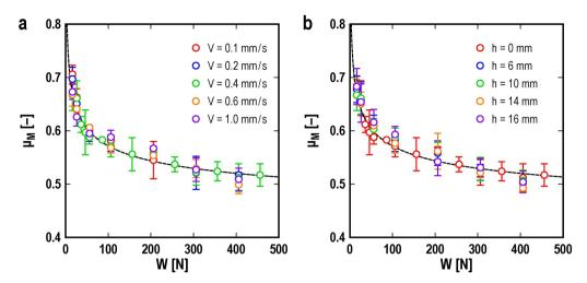
Figure 3 | Macroscopic static friction coefficient  $\mu_{\rm M}$  vs. loading force W. The dependence of the macroscopic static friction coefficient  $\mu_{\rm M}$  on the loading force W is shown for various values of (a) the driving velocity V and (b) the height h. The error bars indicate the standard deviation. In (a), h = 0 mm, and in (b), V = 0.4 mm/s. The broken lines show the results obtained by fitting the data with Eq. (3) for V = 0.4 mm/s and h = 0 mm.
