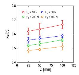
Figure 5 | Macroscopic static friction coefficient  $\mu_{\rm M}$  vs. sliding surface length L'. The dependence of the macroscopic static friction coefficient  $\mu_{\rm M}$  is shown for the length of the sliding surface L', i.e., the apparent contact area. The length of the upper surface of the slider is held constant at  $L=100\,$  mm. The error bars indicate the standard deviation. The experimental parameters are  $V=0.4\,$  mm/s and  $h=0\,$  mm.
