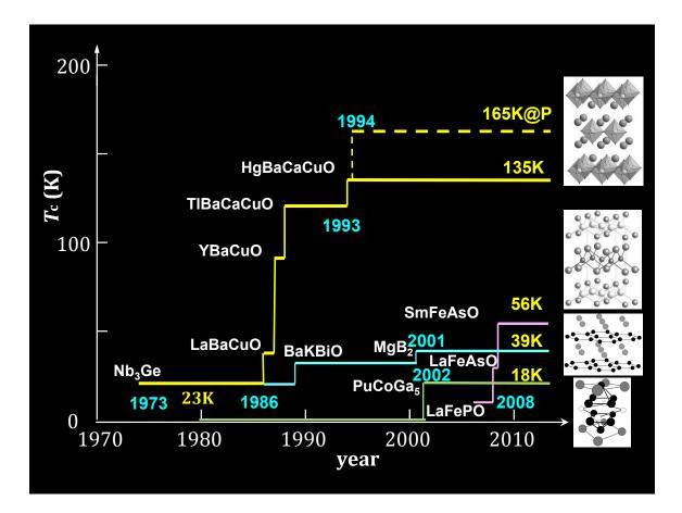
Figure  $1 - T_c$  versus time. Superconducting transition temperatures versus year of discovery for various classes of superconductors. The images on the right are the crystal structures of representative materials.
