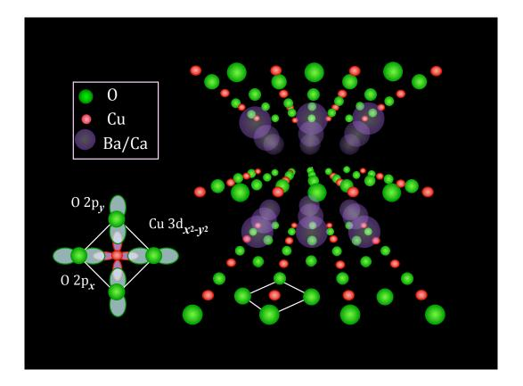
Figure 3 – **Crystal structure.** Layered cuprates are composed of  $CuO_2$  planes typically separated by insulating spacer layers. The electronic structure of these planes primarily involves hybridization of a 3d x<sup>2</sup>-y<sup>2</sup> hole on the copper sites with planar coordinated  $2p_x$  and  $2p_y$  oxygen orbitals.
