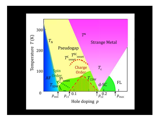
Figure 2 – **Phase diagram.** Temperature versus hole doping level for cuprates, indicating where various phases occur. AF is antiferromagnet, d-SC d-wave superconductivity, and FL Fermi liquid. SDW and CDW represent incommensurate spin density wave and charge density wave order. "onset" marks where precursor order or fluctuations become apparent.
