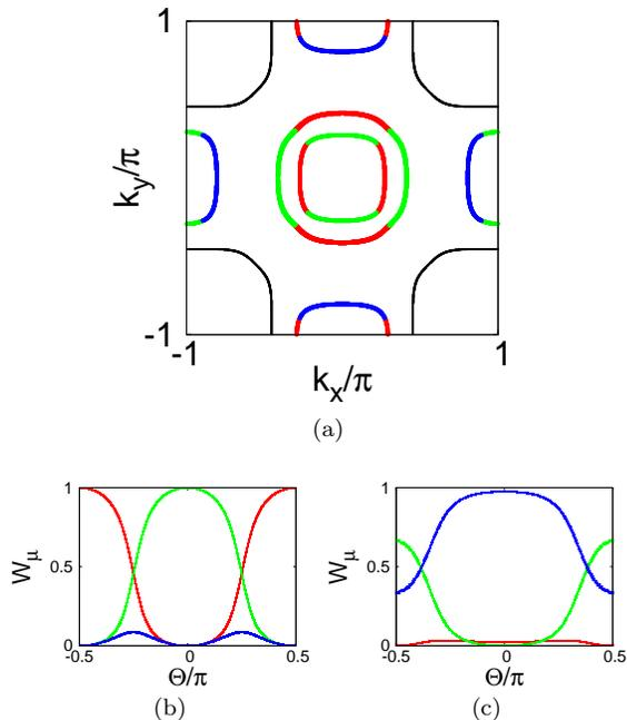
FIG. 5. (a) Fermi surface in the three-orbital model with hopping parameters as given in Table I in the unfolded BZ. The main orbital contributions in (a) are shown by following colors:  $d_{xz}$  (red),  $d_{yz}$  (green), and  $d_{xy}$  (blue). Orbital-weight  $W_\mu$  for the outer hole pocket and electron pocket at  $(\pi, 0)$  in (a) are shown in (b) and (c) respectively. The angle  $\Theta$  is measured from  $k_x$ -axis.
