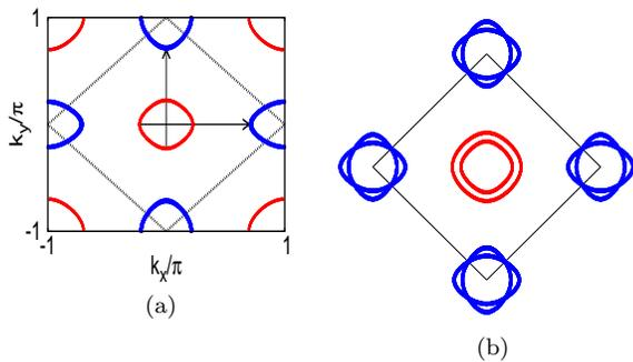
FIG. 2. Fermi surface for the half-filled two band model with  $t_1 = -1.0$ ,  $t_2 = 1.3$ ,  $t_3 = t_4 = -0.85$  in the (a) unfolded (1 Fe atom/unit cell) BZ and (b) folded BZ. The hole and electron pockets are separated by wave-vector  $(\pi, 0)$  and  $(0, \pi)$ , showing Fermi surface nesting.
