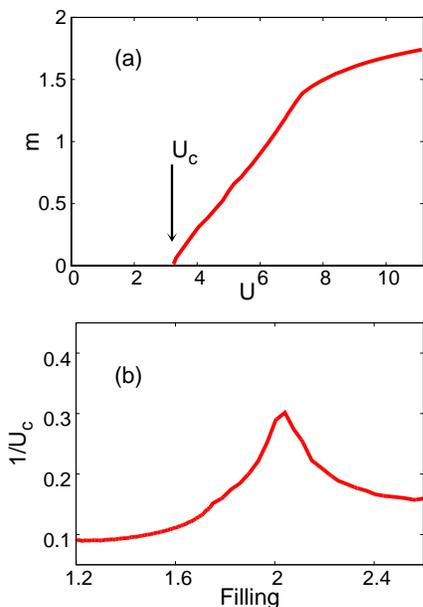
FIG. 3. (a) Variation of sublattice magnetization with  $U$  for  $n \sim 2$  and  $J=0$ , showing onset of  $(\pi, 0)$  magnetic order at critical interaction strength  $U_c \approx 3.0$ . (b) The inverse of critical interaction  $U_c^{-1}$  shows a maximum around electron filling  $n \sim 2$  corresponding to nesting between hole and electron Fermi pockets, showing proclivity of the two-band system towards  $(\pi, 0)$  magnetic ordering.
