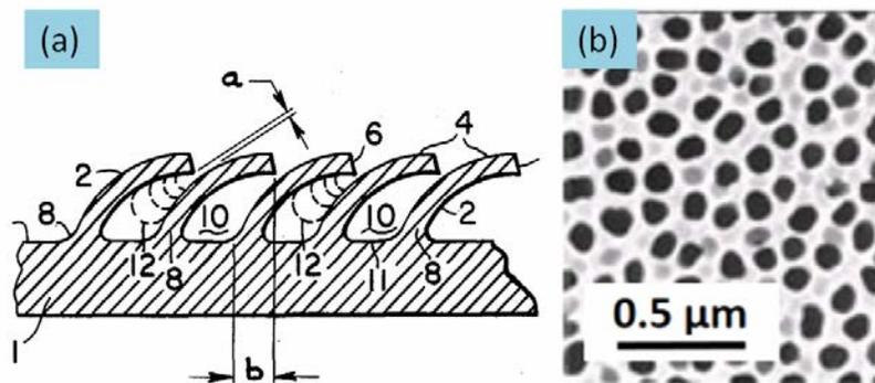
Figure 8. Examples of surface machining and roughening: (a) a machined surface with bent fins to enhance nucleate boiling, from patent<sup>118</sup>; gap  $a$  is in the 25-125  $\mu\text{m}$  range; (b) electrochemically processed porous alumina (Anodisc™).
