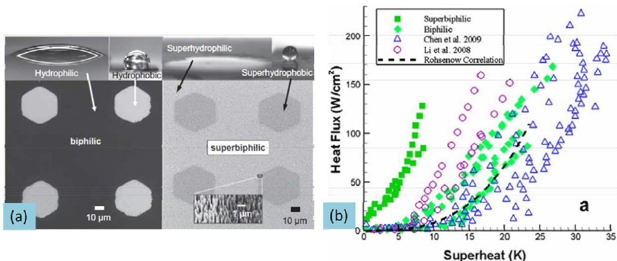
Figure 18. Biphilic and superbiphilic patterns (a) on silicon surfaces drastically enhance pool boiling heat transfer (b) Reprinted from<sup>58</sup>, Copyright 2013, with permission from Elsevier.
