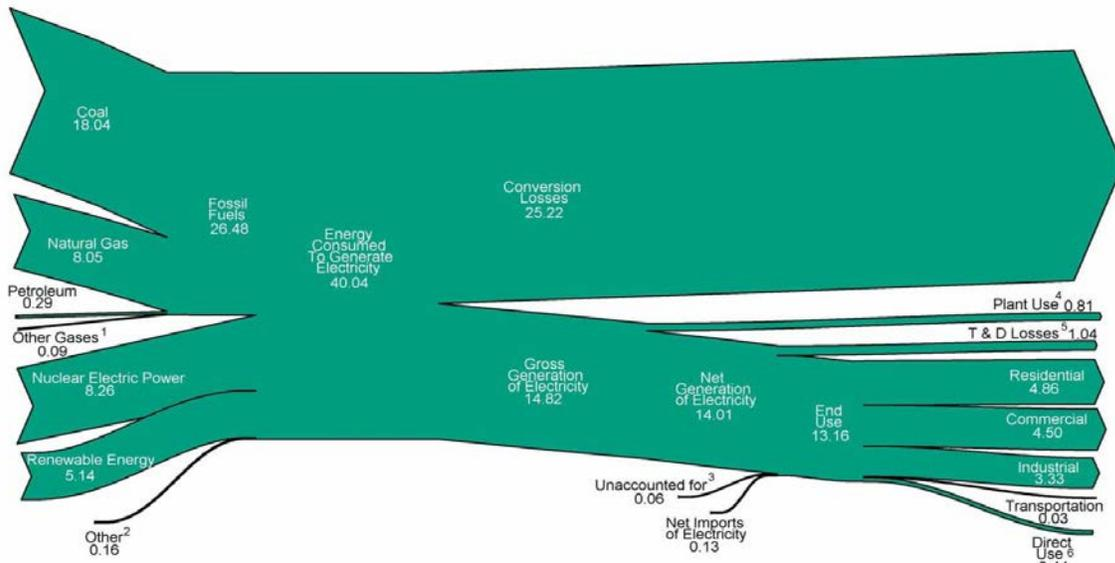
Figure 22. US electricity flow, in Quad, from production source to consumption sectors, year 2011. See <sup>338</sup> for original image and detailed caption. One Quad (quadrillion BTU) equals  $10^{15}$  BTU or approximately  $10^{18}$  Joule.
