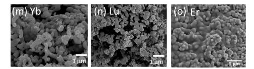
Fig. 6 (a-n) SEM micrographs of (RE)CrO<sub>3</sub> powders. (o) ErCrO<sub>3</sub> pellet after densification sintering at 1300° C for 15 hours.
