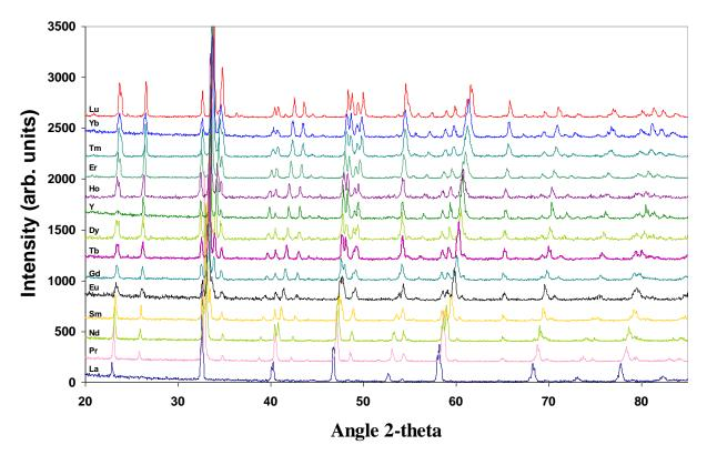
Fig. 3 XRD patterns of (RE)CrO<sub>3</sub> powders. The diffraction peaks move to higher angles with decreasing lattice plane spacing.
