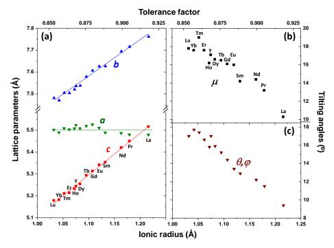
Fig. 4 (a) Lattice parameters a, b and c vs the RE ionic radius and the perovskite tolerance factor. The increase of b and c with IOR implies an increasing unit cell size. (b,c) The decrease of  $\theta$ ,  $\varphi$  and  $\mu$  with IOR implies decreasing tilting of the perovskite octahedra.
