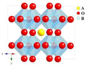
**Fig. 1** 8 unit cells of the ideal cubic ABO<sub>3</sub> perovskite structure showing the 12-fold coordination of the A-site cation and the 8-fold octahedral coordination of the B-site cation.
