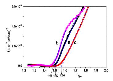
Fig. 7: Graphs of  $(\alpha hv)^2$  Vs hv for CdTe thin films made by (a) conventional, (b) rotating shutter and (c) rotating cylinder methods
