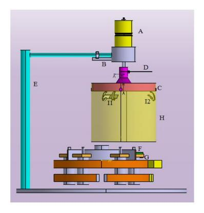
Fig. 1: schematic of a new vapor controller system; (A) dc motor, (B) motor holder, (C) revolving disk(shutter), (D) substrate, (E) stand, (F) boat, (G) electrode, (H) cylinder, (II I2) two extra substrate holders
