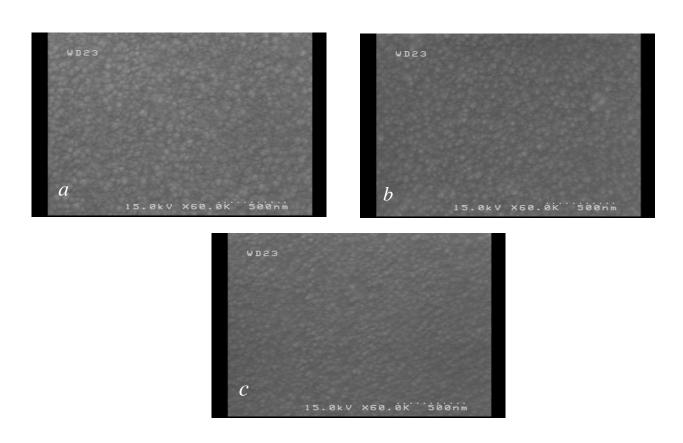
Fig. 5: the surface morphology of the CdTe thin films made by (a) conventional, (b) rotating shutter system and (c) rotating cylinder methods
