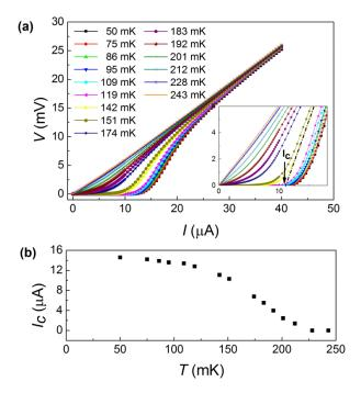
**FIG.2** (Color online) (a) Temperature-dependent *V-I* characteristics of the 5-uc (110) LaAlO<sub>3</sub>/SrTiO<sub>3</sub> interfaces measured at different temperature. The insert shows that the critical current ( $I_c$ ) was gained by extrapolating the linear part near the upward corner of the *V-I* curves to zero axis. (b) Temperature dependence of the  $I_c$  obtained from (a).
