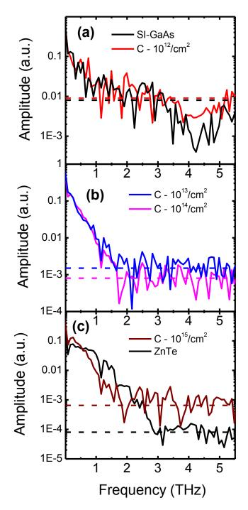
**Figure 4.** FFTs of the THz pulses recorded from different carbon irradiation dose photoconductive antennas. The dotted lines are indicating the noise level.
