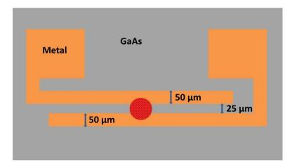
**Figure 1.** Schematic diagram of the electrodes on a photoconductor used for THz pulse detection. The THz pulse to be detected will be focused on the same spot of optical carrier excitation with almost matching arrival time of the 800 nm pulse. The photogenerated charge carriers will move in the presence of the electric field of the THz pulse and a current flow will be measured at the
