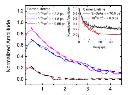
**Figure 2.** Optical NIR time resolved pump-probe reflection curves of non-irradiated and irradiated SI-GaAs. The dash-lines are fits to a single exponential decay. The inset shows the non-irradiated sample with mostly a slow fall ( $\sim$ 70 ps), except for the beginning of the signal, while the low irradiated sample exhibits already a comparatively rapid decay ( $\sim$ 6 ps).
