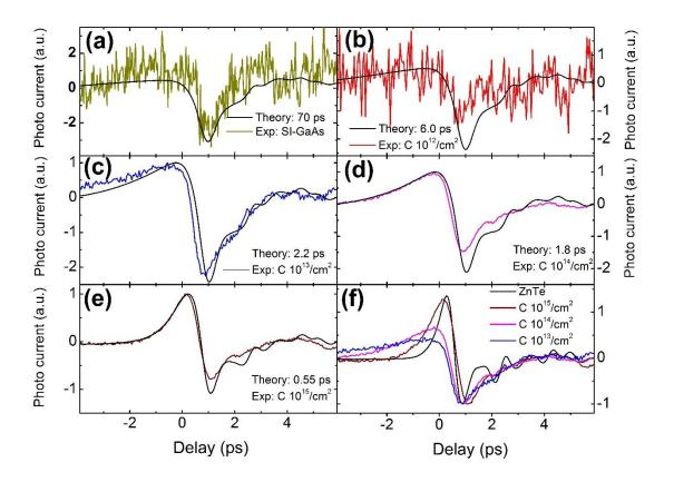
**Figure 3.** THz pulses recorded from different carbon irradiation dose photoconductive antennas (PCAs) with their theoretically predicted pulse shapes (a-e). In (f) the THz pulse shape recorded from the 3 highest dosages PCA detector is plotted together with the pulse shape recorded from the ZnTe electro optic crystal (continuous black curve).
