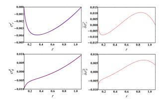
FIG. 4: (a)  $\sigma_r^r$  as a function of r for a surface of positive constant reference Gaussian curvature. The parameters are  $r_{in} = 0.1$ ,  $r_{out} = 1.1$  and  $\sqrt{k_G} = 1/4$ . We compare the exact solution (solid blue line, obtained numerically) to our first-order approximation (red dashed line). (b) Normalized deviations of our first-order approximation
