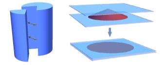
FIG. 2: An illustration of the geometry and the stressed state of a disclination. The stressed state of a 3D material containing a disclination on a cross-section (left panel) is identical to that of a flattened cone (right panel).
