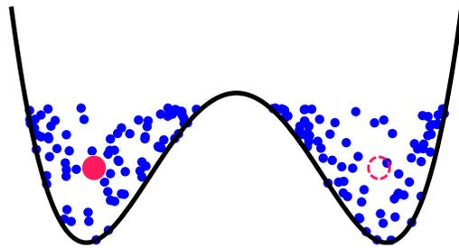
FIG. 1: (Color online) Schematic of the proposed set-up. A bosonic Josephson junction consists of  $N$  identical bosons (represented by the small blue dots) which are able to tunnel between the two sides of a double well potential. To this is added a single impurity atom (large red dot) which is also able to tunnel between the two wells.
