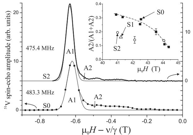
FIG. 9:  $^{51}\text{V}$  NMR spectra at  $T = 380$  mK for samples S0 and S2 measured at 483.3 and 475.4 MHz, respectively. Solid lines show the fitting results of the main peak of the spectral pattern with a Lorentzian line (A1). Inset: Relative integral intensity of the residual contribution A2 of the NMR spectra pattern which does not belong to the main line A1. Data from different samples S0 (solid squares), S1 (open triangle), and S2 (open circles) are shown.
