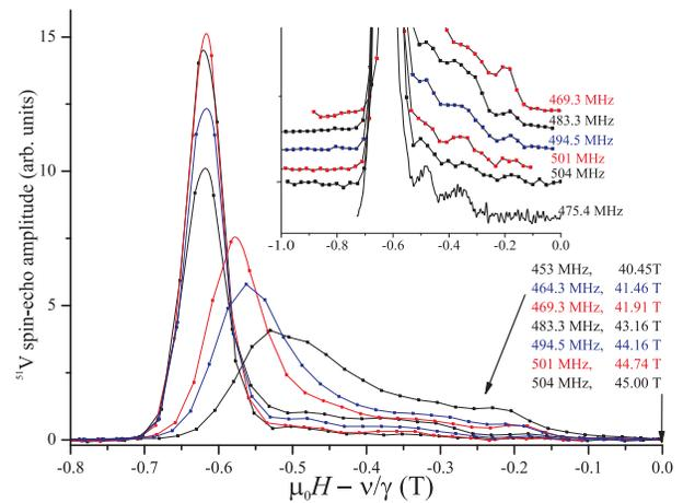
FIG. 8:  $^{51}\text{V}$  NMR spectra of sample S0 obtained at  $T = 380$  mK for different applied magnetic fields in the range  $40.45 < \mu_0 H < 45$  T. Inset: Data for sample S2 are plotted additionally (solid line). The base lines of the different spectra in the inset are shifted along the  $y$ -axis for better visibility.
