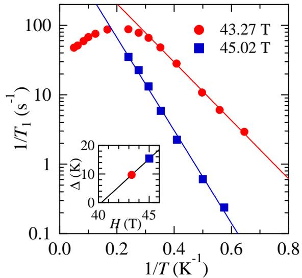
FIG. 4: Temperature dependence of the spin-lattice relaxation rate  $1/T_1$  at  $^7\text{Li}$  nuclei in Arrhenius representation measured for different applied magnetic fields  $\mu_0 H = 43.27$  T and  $45.02$  T. Inset: The slopes of the Arrhenius representations, i.e. activation energies  $\Delta$ , plotted vs. the applied magnetic field  $H$ . The solid line indicates a linear fit (see text).
