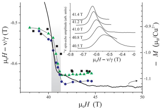
FIG. 3: Peak positions of the  $^{51}\text{V}$  NMR spectra in  $\text{LiCuVO}_4$  are plotted against applied field along the  $c$ -direction obtained from samples S0 (squares), S1 (triangles), and S2 (bullets), respectively (left axis). The solid line shows the bulk magnetization  $M(H)$  vs. the applied magnetic field  $H$  obtained from sample S0\* (right axis). Inset:  $^{51}\text{V}$  NMR spectra of sample S2.
