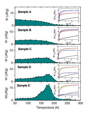
Figure 4: Magnetic work defined as the area enclosed by the increasing and decreacing magnetic field curves as function of temperature for different samples. In the insets we show magnetization loops at 250 K (black), 170 K (red) and 60 K (blue).
