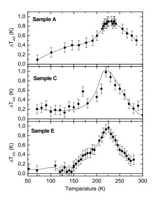
Figure 3: Adiabatic temperature change ( $\Delta T_{AD}$ ) for samples A, C and E as function of temperature when the magnetic filed is increased from 0 to 3 T. The values of  $\Delta T_{AD}$  where extracted from DTA measurements taking into account the heat exchange between the sample and the sample holder.
