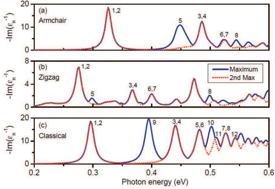
Figure 1: The eigenvalue loss spectrum  $-\text{Im}[\epsilon_n^{-1}(\omega)]$  in equilateral graphene triangles of sidelength 20 nm. Each peak defines a plasmon mode (labeled by  $n = 1, 2, 3, \dots$  in order of decreasing imaginary part), and the coincidence of the maximum (blue solid) and the second maximum (red dotted) indicates the energy degeneracy. Results of the quantum tight-binding method in (a) for armchair edges, and in (b) for zigzag edges, while classical results are given in (c).
