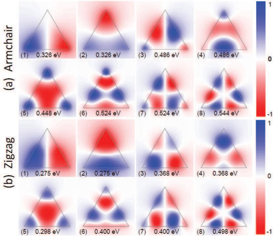
Figure 3: In-plane potential  $\phi_n$  extracted from the eigenvalue loss spectrum calculations. (a) The lowest 8 plasmon modes in an armchair triangle; (b) the corresponding plasmon modes in a zigzag triangle.
