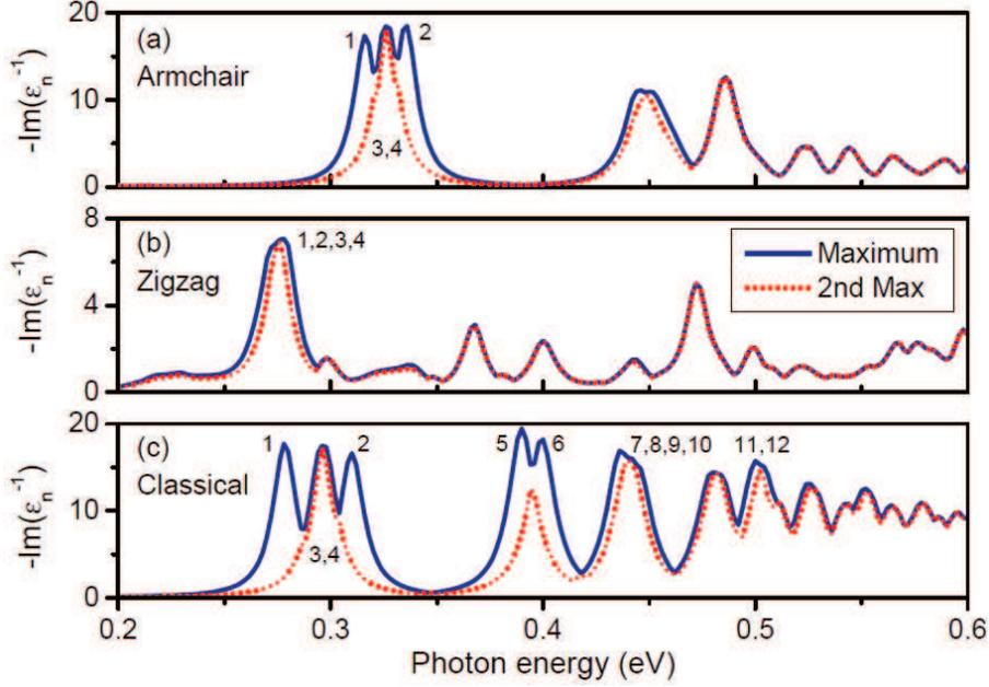
Figure 4: The eigenvalue loss spectrum  $-\text{Im}\epsilon_n(\omega)^{-1}$  in graphene bow-tie triangles with gap width 0.5 nm. Results obtained from quantum calculations in armchair triangles (a) and in zigzag triangles (b) are compared with classical calculations in (c).
