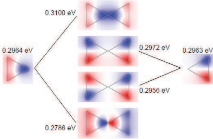
Figure 5: A schematic diagram of the dipole mode hybridization in classical calculations. There is a larger energy splitting for  $x$ -polarized dipole, and the antisymmetrically coupled modes have lower energy for both polarizations. Here the gap distance is 0.5 nm.
