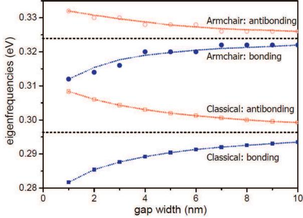
Figure 6: The eigenfrequencies of the hybridized modes as a function of gap width for  $x$ -polarized dipoles in classical calculations and armchair triangles, respectively. The two dotted lines (0.296 eV and 0.324 eV) are the dipole eigenfrequencies associated with the individual triangles.
