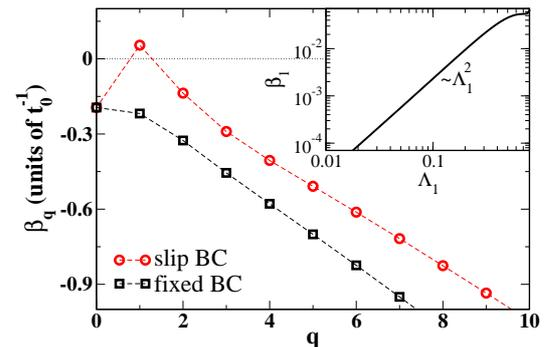
FIG. 3: Dispersion relation for the shear-free (slip BC) and the Dirichlet (fixed BC) boundary condition. Parameters are  $\bar{\Lambda}_1 = 0.7$ . The time scale is  $t_0 = l_0/(MkR_0^2)$ . The inset shows the positive growth rate  $\beta_1$  depending on the radial layer number  $\Lambda_1$ .
