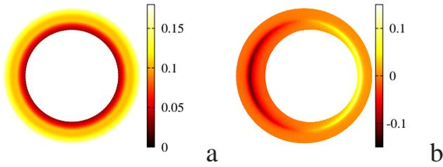
FIG. 4: Network shape before (a) and after symmetry-breaking (b). (b) was obtained by superimposing the axisymmetric shape and the unstable mode with the amplitude  $0.15 \Lambda_1$ . The color encodes the spatial distribution of the strain energy density (a) and the change in strain energy density (b). The energy density scale is  $k/l_0$ .
