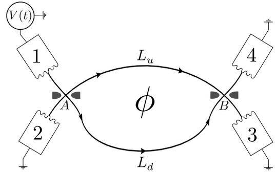
FIG. 1. Mach-Zehnder interferometer driven by a time dependent voltage  $V(t)$ . The interferometer consists of two paths of lengths  $L_u$  and  $L_d$  which enclose a magnetic flux  $\phi$ . Two quantum point contacts  $A$  and  $B$  allow the single particle states to be delocalized over both paths leading to interference contributions in current and noise measured at the outputs.
