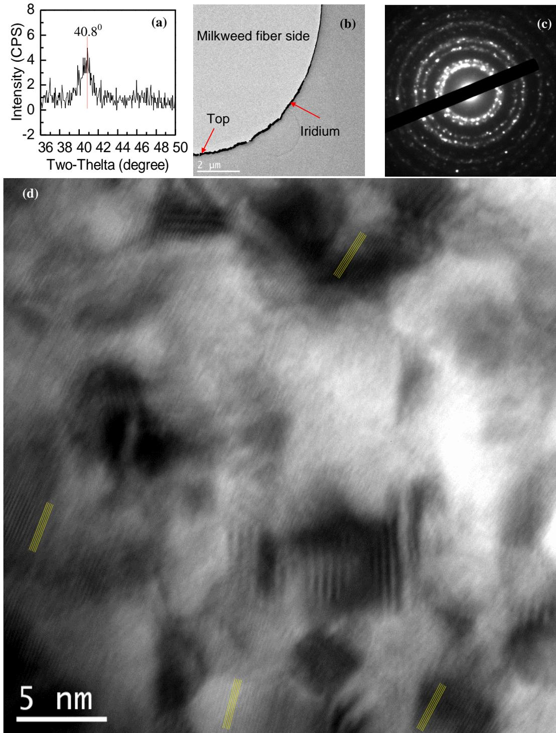
FIG. 6. (a) XRD pattern of 10 layers of 3.2 nm-thick Ir films on milkweed fibers. The peak appears at  $40.8^\circ$ , which indicates that the Ir film is composed of crystals. The crystalline size is
