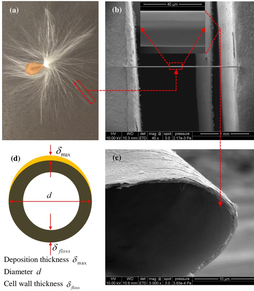
FIG. 1. (a) A milkweed seed and floss. (b) SEM image of a single milkweed fiber suspended across two electrodes (the long sample). The inset shows the floss surface. (c) SEM image of the milkweed fiber cross section. (d) Profile of the milkweed fiber cross section coated with a layer of Ir, and the definition of maximum thickness  $\delta_{\max}$ . The average thickness of the Ir film is
