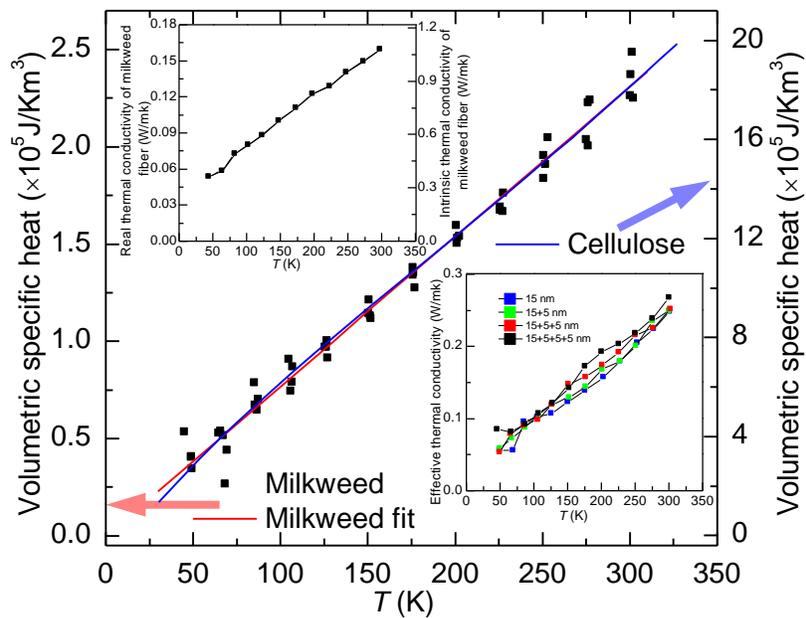
FIG. 4. Temperature dependent volumetric specific heat of milkweed and microcrystalline cellulose. The inset in the upper left corner shows the effective and intrinsic thermal conductivity of the milkweed fiber. The inset in the bottom right corner shows the effective thermal conductivity of the Ir-coated milkweed fiber.
