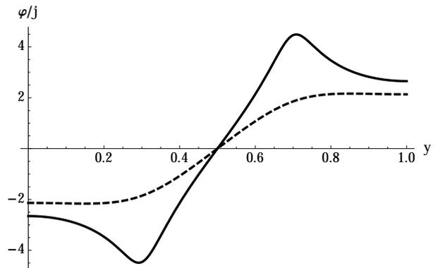
FIG. 4. The phase  $\varphi(x_0, y)$  for  $j = 1$  at fixed distances  $x_0$  from the edge  $x = 0$  as a function of the transverse coordinate  $y$  for symmetric contacts at  $y_1 = 0.3$  and  $y_2 = 0.7$ . The solid line is for  $x_0 = 0.05$ , the dashed line is for  $x_0 = 0.2$ .
