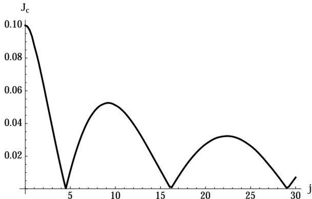
FIG. 6.  $J_c(I/I_0)$  for the junction width  $\Delta x = 0.1$  and symmetric contacts at the edge  $x = 0$  and  $y_1 = 0.48$  and  $y_2 = 0.52$  so that the distance between contacts is  $\Delta y = 0.04$ .
