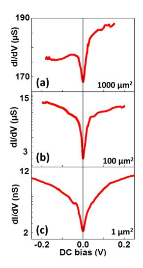
Figure 2. Voltage dependence of the differential conductance for three vertical Ni/Graphene/MgO/Co spin-valves with junction area of 1000  $\mu$ m<sup>2</sup>(a), 100  $\mu$ m<sup>2</sup>(b) and 1  $\mu$ m<sup>2</sup>(c), at 1.5 K.
