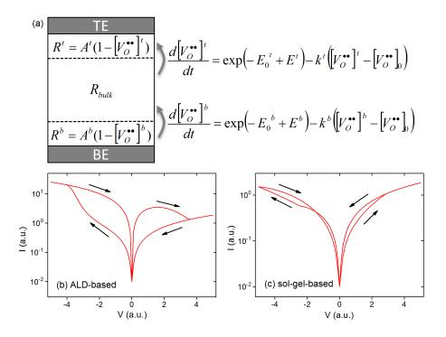
**FIG. 3.** (a) Scheme of the proposed model for the resistive switching mechanism. In the ALD-based devices the movement of oxygen ions only occurs in the proximity of the top electrode, whereas in the sol-gel-based devices occurs in both interfaces. Numerical simulations showing a qualitative matching with the experimental I-V curves for (b) the ALD-based devices and (c) the sol-gel-based devices. The arrows indicate the path of the applied voltage sweep.
