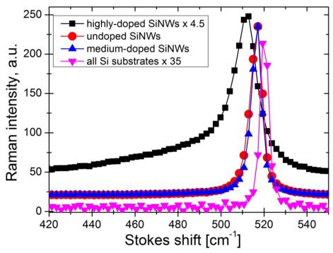
**Figure 8.** Raman spectra of silicon nanowire ensembles prepared from silicon substrates with three different doping levels. The spectrum of a silicon substrate, with the zone-center optical phonon line at  $520 \text{ cm}^{-1}$ , is shown for comparison.
