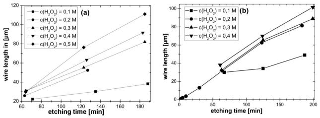
**Figure 2.** Length of the silicon nanowires as a function of the etching time for different concentrations of the oxidizing agent H<sub>2</sub>O<sub>2</sub>. (a) Undoped silicon (100), specific resistivity  $\rho > 1000$   $\Omega$ cm. (b) Medium boron-doped silicon (100) ( $\rho = 14-23 \Omega$ cm), *p*-type.
