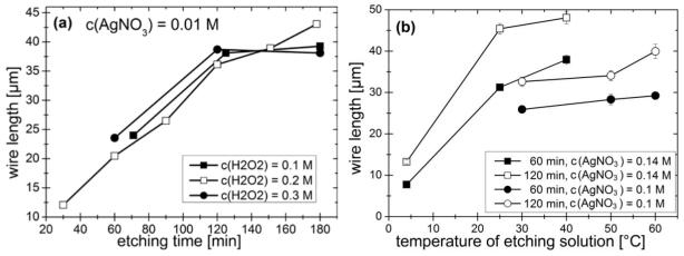
**Figure 3.** Length of the silicon nanowires obtained from highly doped silicon (100) ( $\rho < 0.01 \ \Omega cm$ ) as a function of the etching time for different concentrations of the oxidizing agent H<sub>2</sub>O<sub>2</sub> (**a**) and as a function of etching temperatures for different silver nitrate concentration (**b**). There seems to be a saturation value so that the lengths of the wires are limited to about 50 µm.
