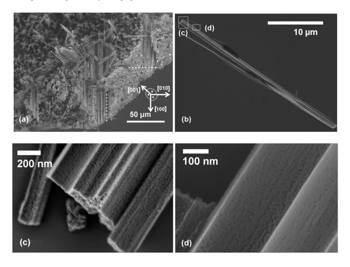
**Figure 4.** (a) Medium boron-doped Si ( $\rho = 14-23 \ \Omega cm$ ), etched for t = 2 h,  $c_{\text{H2O2}} = 0.2 \text{ M}$ ,  $c_{\text{HF}} = 4.8 \text{ M}$ . SEM image of a slightly tilted silicon wafer after the etching illustrating the etching
