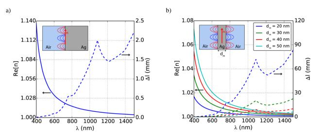
Fig. 2. The effective mode index real part Re[n] (solid lines) and propagation distance  $\Delta l$  (dashed lines) of SPPs at air-silver interface (a) and of long-range SPPs at air-silver-air structure (b). The  $d_m$  denotes the thickness of the silver film and  $\lambda$  is the wavelength of light. The structure under investigation is also presented in the inset.
