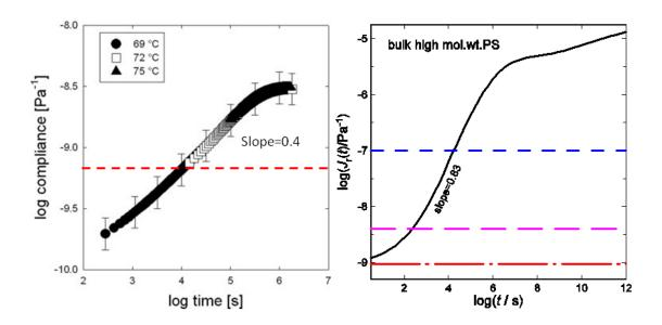
Fig, 2. (a) Master curve constructed from data of the 36 nm thick PS film shown in Fig.1 (data from Ref.[34] are redrawn). (b) Master curve constructed from the recoverable shear creep compliance  $J_r(t)$  data of 600,000 Da bulk PS taken at temperatures above  $T_g$ =100 C by Plazek and O'Rourke Ref.[22]. The horizontal lines show the bounds of the contributions from the segmental  $\alpha$ -relaxation and the sub-Rouse modes according to Eqs.(1) and (2).
