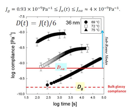
Fig.1. Creep compliance curves for a 36 nm thick PS film at temperatures of 69, 72, and 75.8 C. Data from Ref.[ 34] redrawn.
