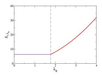
FIG. 3: (color online) Critical repulsive interaction coupling constant  $g_{c,\lambda_R}$  as a function  $\lambda_R$ . The dashed vertical line separates the regimes of constant and variable  $g_{c,\lambda_R}$ . Units are specified in the text.
