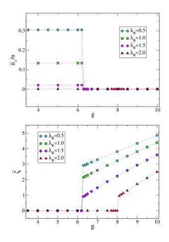
FIG. 1: (color online) Optimal variational parameters  $\bar{n}_+$  and  $\bar{\zeta}$ , plotted in function of g for different values of  $\lambda_R$ . Units are specified in the text.
