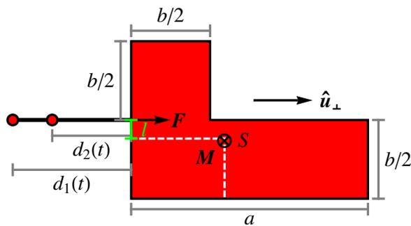
**Figure 1.** Schematic of a force-free and torque-free L-shaped Golestanian-like microswimmer of size  $a$  and orientation  $\hat{\mathbf{u}}_{\perp}$ . To put the microswimmer in motion, the distances  $d_1(t)$  and  $d_2(t)$  of the two small spheres from the L-shaped particle vary as a non-reciprocal function of time. The effective lever arm  $l$  relates the effective force  $\mathbf{F}$  to the effective torque  $M = \|\mathbf{M}\|$  on the centre of mass  $S$ .
