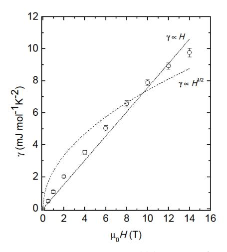
FIG. 5. The *H* dependence of  $\gamma_{\nu}(H)$  as obtained in a "global" fit to the data for  $2 \le T \le 12$  K in 10 fields,  $0 \le \mu_0 H \le 14$  T. The solid and dashed lines represent least-squares fits to *H* and  $H^{1/2}$  dependences (see text). The error bars correspond to the uncertainties determined in the fit.
