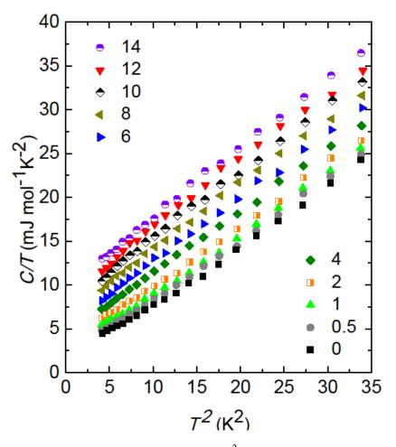
FIG. 4. (Color on line) The specific heat as C/T vs  $T^2$  to 6 K in 10 fields,  $0 \le \mu_0 H \le 14$  T. The deviations from linearity suggest the presence of a low concentration of paramagnetic centers.
