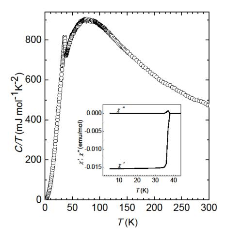
FIG. 1. The specific heat in zero field, as C/T vs T, for 2 - 300 K. The superconducting transition is marked by the sharp peak in C/T near  $T_c = 36.9$  K. At that temperature, as shown in the inset, the ac susceptibility shows a sharp and complete transition to the superconducting state.
