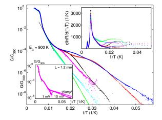
Figure 1: (Color online)Temperature dependences of dark ohmic conductance, G(T), normalized to its room-temperature values,  $G_{300}$ , for different *m*-TaS<sub>3</sub> samples. Top inset shows corresponding temperature derivatives of the resistance,  $d \ln R/d(1/T)$ . Bottom inset shows G(T)curves measured at various sample voltages for the sample marked by magenta color in the main figure.
