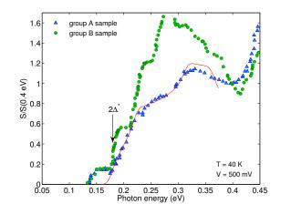
Figure 5: Photoconduction spectra of the samples of the groups A and B. Solid curve shows the best fitting by the Peierls gap modulation model [13].
