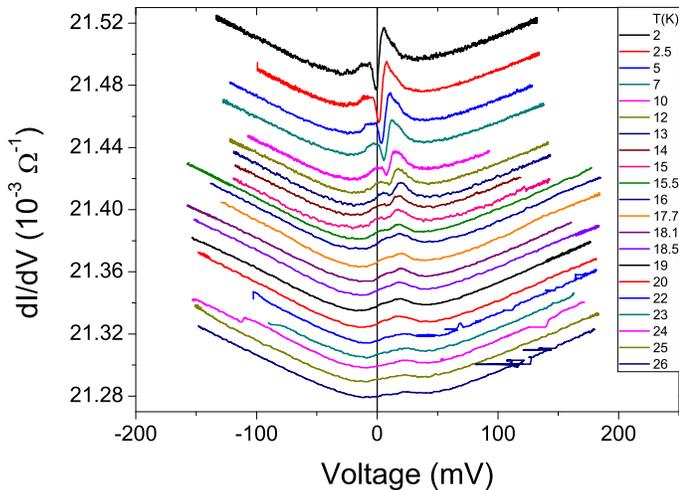
FIG. 2. (Color online) Differential conductance of a tunnel junction in the  $c$  direction taken from 2 to 26 K. Note the reduction of the predominant sharp characteristics close to the Fermi level when the temperature is increased. The minimum is displaced from the origin to positive bias voltage. Raising the temperature the structure is smoothed. At high bias voltages the background of the tunnel junction looks normal. All data was vertically displaced for a clear view.
