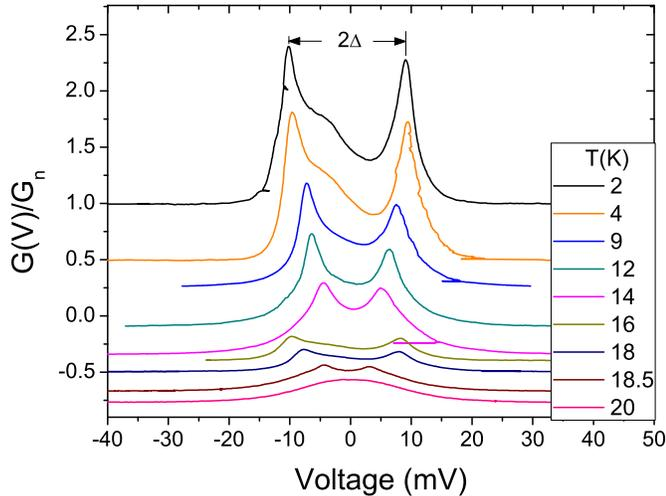
FIG. 4. (Color online) Normalized differential conductance of a tunnel junction measured in the  $a$  crystallographic direction. These curves show the presence of a bigger distortion, different to the observed in  $c$  crystallographic direction. Note that the structure of the Fano resonance is distorted with two symmetrical peaks at  $\pm 10$  mV. The features decreases as the temperature rises, at 14 K the feature look similar to a contact junction with a  $Z$  parameter about 0.2 [42].
