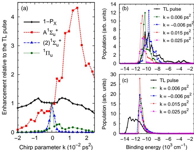
FIG. 2: Theoretical results ( $I_{TL} = 7.2 \times 10^{12} \text{ W/cm}^2$ ) for: (a) Chirp dependence of the total photoassociated population ( $1 - P_X$ ) and the final populations in the states of the probed UV-emitting band. (b) Final vibrational distribution in the intermediate  $(1)^1\Pi_g$  state for various values of the chirp parameter  $k$ . (c) Same as in (b) but obtained within a reduced model comprising only the  $X^1\Sigma_g^+$  and  $(1)^1\Pi_g$  states.
