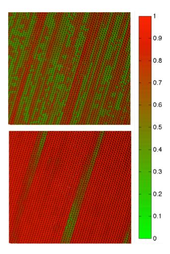
**Fig. 8** Snapshot of the distorted crystal phase for the system of N = 3600 COs at  $P^*=59.4$ . (Top Panel) Particles are colored with respect to the local value of  $\varphi_4^j$ . (Bottom Panel) Particles are colored with respect to the local value of  $\varphi_6^j$ .
