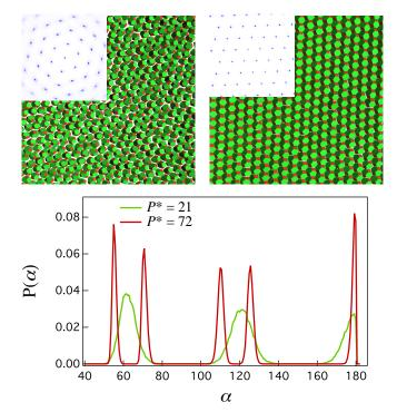
**Fig. 10** (Top Panel) Representative snapshots and corresponding structure factors for a system of N=1600 TOs at (left)  $P^*=21$  (hexagonal rotator phase) and (right)  $P^*=72$  (rhombic phase). (Bottom Panel) Probability density function of angle,  $\alpha$  for a system of N=1600 TOs at the same two pressures.
