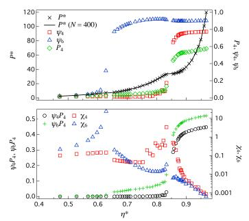
**Fig. 9** Equation of state for 1600 TOs obtained by expansion runs. Legend as in Fig. 1. The value of  $\eta^{crys}$  is estimated as 1.05.
