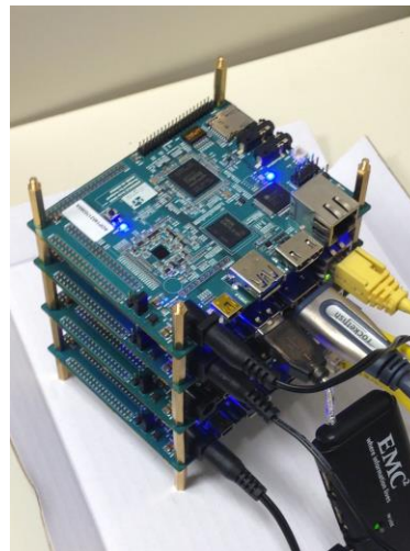
Figure 7 – The Octa-Cluster under construction with 4 servers
