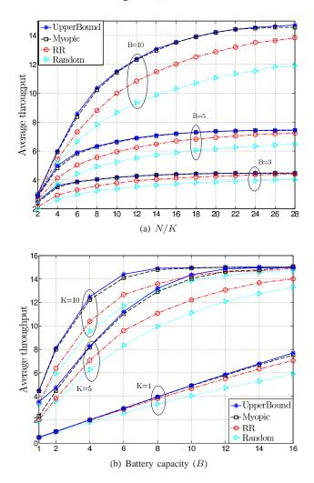
Figure 2. (a) Average throughput vs. number of nodes, N, with K = 5 channels, and battery capacity B = 3, 5, 10, and (b) average throughput vs. battery capacity, N = 30, and K = 1, 5, 10.
