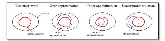
Figure 5: Static Analysis is an approximative approach
