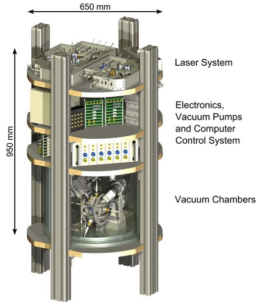
**Figure 1.** CAD model of the experimental setup. The assembly consists of four platforms, each with a diameter of approximately 65 cm. From top to bottom, they are used for the laser system, vacuum pumps, computer control system and electronics, and the vacuum chambers.
