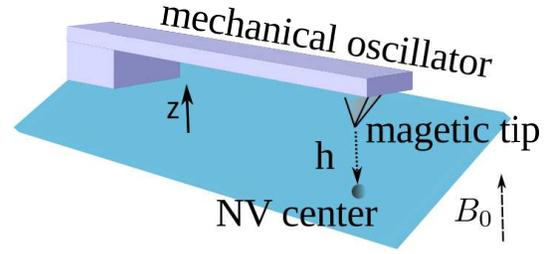
**Figure 2** A magnetic tip, which is attached to the end of a cantilever, is placed at a distance  $h$  above a single NV center. It creates a strong magnetic gradient near the electronic spin of the NV center. As the spin energy is in proportional to the magnetic field, a strong coupling between the NV center electrons spin and the motion of cantilever is created. Laser field is used for initializing and measuring the spin states. Microwave is used for manipulating the spin states.
