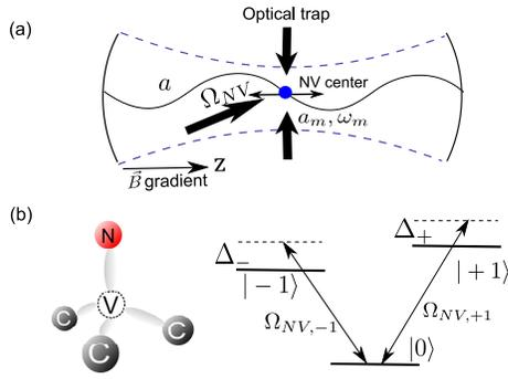
**Figure 9** (a) A nanodiamond with a NV center is optically trapped in vacuum with spin-mechanical coupling enabled through a nearby magnetic tip and opto-mechanical coupling through a cavity around. (b) The atomic structure (left) and the level diagram (right) in the ground state manifold for a NV center in the nanodiamond. Figure adopted from [50]. Copyright (2013) by The American Physical Society.
