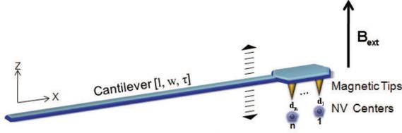
**Figure 4** A scheme to entangle multiple NV centers spins that couple with the same mechanical oscillator. (a) An array of evenly spaced magnetic tips are attached at the end of a nanomechanical cantilever, under which are one-to-one correspondent NV centers. Figure adapted from Ref. [57]. Copyright (2010) by The American Physical Society.
