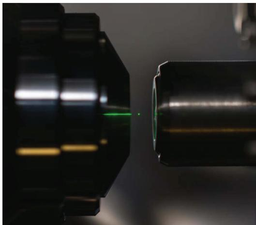
**Figure 12** A photograph of a  $\sim 100$  diameter nanodiamond which is levitated by an optical tweezer (1064 nm). The green color is from an optical pump 532 nm laser. The trapping lens is on the left, and the lens on the right is used to collimate the light exiting the trap. Figure adopted from [46]. Image credit: J. Adam Fenster, University of Rochester.
