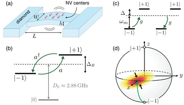
**Figure 7** (a) All-diamond doubly clamped mechanical resonator with an embedded NV centers ensemble (NVE). (b) Spin levels and transitions of NV centers electron spins. Local perpendicular strain induced by beam bending mixes the  $|\pm 1\rangle$  states. (c) NV centers spins in the two-level subspace  $|\pm 1\rangle$  off-resonantly couple with a common mechanical mode. (d) NVE collective spins squeezing. Figure adapted from Ref. [37]. Copyright (2013) by The American Physical Society.
