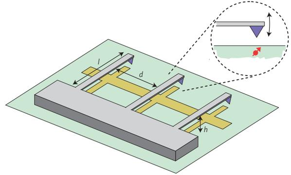
**Figure 5** Schematic view of a scalable quantum information processor on an electromechanical quantum bus and NV centers spins as qubits. Figure adapted from Ref. [30]. Copyright (2010) by Nature Publishing Group.
