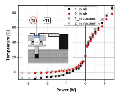
**Figure 3**: Temperature of the cell as a function of power in air and under vacuum: T1 refers to thermocouple 1 that placed on the cooper plate directly connected to the thermoelectric element. T2 represents the second thermocouple which measured the temperature on the membrane supporting mesh (closest position to the sample).
