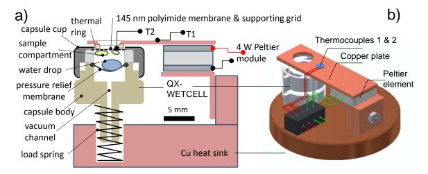
**Figure 2**: Schematic drawing of the 4.2 W thermoelectric cooling / heating setup for QuantomiX WETSEM capsules (see details in the text).
