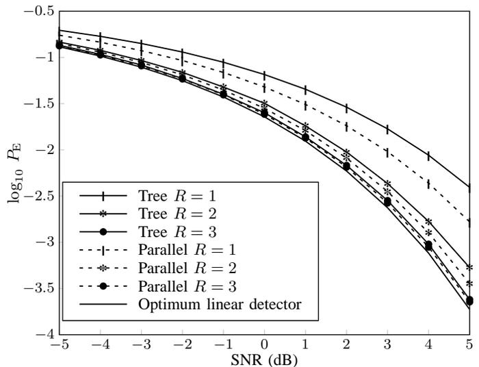
Fig. 6. Comparison of error probability performance of the designed tree network with rate pairs  $(R, R)$  and parallel network with rate  $R$ .
