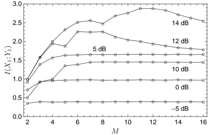
Fig. 3. The mutual information according to Theorem 4 for  $M$ -PSK constellations with uniform probabilities, for the indicated values of  $P_1/P_{\text{ase}}$ . The peak of each curve yields the lower bound in Fig. 2 (c).
