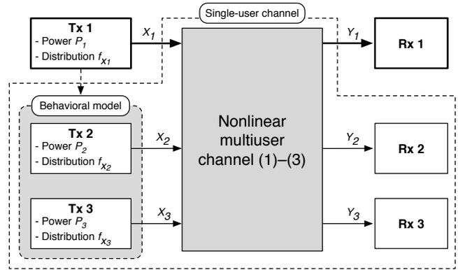
Fig. 1. A single-user channel model can be seen as a combination of a multiuser channel model and a behavioral model for all users but one. Transmitter and receiver are marked Tx and Rx, respectively.
