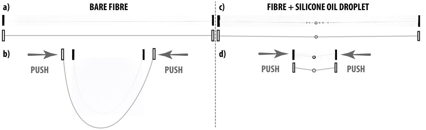
Figure 5: **Artificial spider capture thread.** Left: a thin micrometer-sized TPU filament is held on a caliper. Bringing the ends together leads the filament to exhibit a characteristic catenary-like sagging shape (note: the outlines serve as guides for the eye). Right: This behaviour changes after deposition of a small silicone oil droplet on the filament: bringing the extremities closer leaves the filament taut while the excess filament enters the central droplet.
