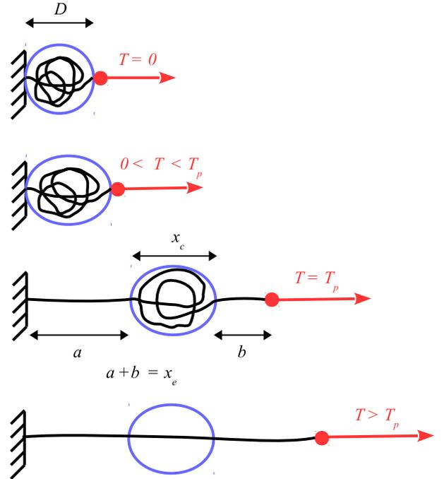
Figure 6: **Two phase model.** The windlass system comprises two phases. The extended phase consists of the fiber that lies outside the drop(s). The coiled phase consists of the fiber that is coiled inside the drop(s). Each phase has its own extension, and there is a fraction  $\rho$  (resp.  $1 - \rho$ ) of the complete fiber is the extended (resp. coiled) phase.
