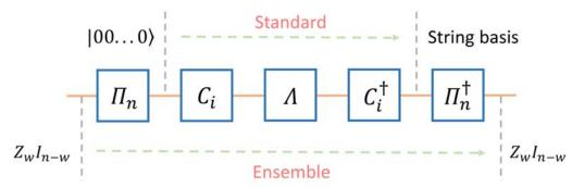
Fig. 1 Quantum circuit to implement the twirling protocol for the purpose of quantum memories. The standard one requires one input state  $|00...0\rangle$  and conjugation by  $C_i$ , whereas the ensemble one requires *n* distinct input states and an additional permutation  $\pi_n$ .
