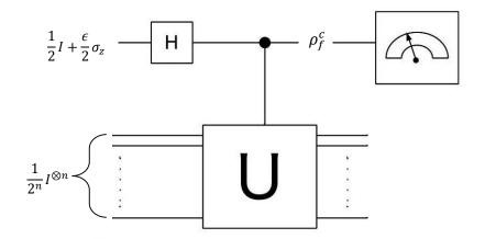
Fig. 8 The DQC1 circuit for evaluating the normalized trace of a unitary matrix with  $2^n$  diagonal elements. The output state shown by Eq. (23) on the control qubit is measured to estimate the normalized trace of U. This task is believed to be computationally hard for a classical computer.
