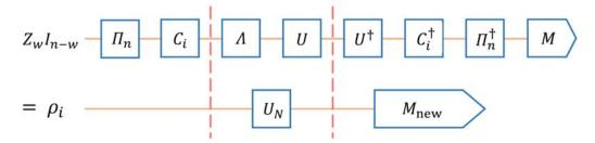
Fig. 2 Quantum circuit for modified twirling protocol to certify noisy Clifford gates. An identity process  $U^{\dagger}U$  is inserted to generate the aim  $U_N$ .  $\rho_i = C_i \pi_n (Z_w I_{n-w}) \pi_n^{\dagger} C_i^{\dagger}$  is a random Pauli state and  $M_{new} = U C_i \pi_n M \pi_n^{\dagger} C_i^{\dagger} U^{\dagger}$  is an efficiently pre-computed Pauli operator if U is a Clifford gate.
