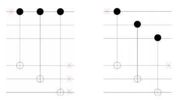
Fig. 5 Two different ways to implement a CNOT gate between the two three-qubit codes: the example on the left is an example of a bad implementation of a CNOT gate between the two three-qubit codes. An error on the first qubit of the first block can propagate to all the qubits in the second block. On the contrary, the right example propagate to at most one error on the bottom encoded qubit and thus remains correctable.
