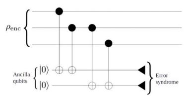
Fig. 3 To detect the error in the encoded state, the ancilla qubits are used to obtain information about the error. Subsequently, the error syndromes can be used to detect and identify the errors. With this knowledge, we can recover the state by applying appropriate recovery operation to the erroneous state.
