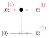
Fig. 4 A bad propagation of errors. An error in the control qubit propagates to the target qubit as well.
