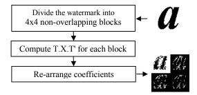
Figure 2. Binary wavelet decomposition process.
