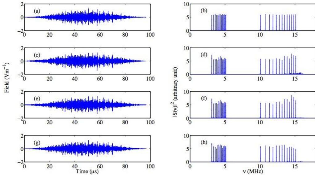
FIG. 4 Optimum fields and their spectrum  $|S(\nu)|^2$  in arbitrary units for the preparation step and the simulation of the elementary transformation  $U_s(\Delta t)$ . Panels (a) and (b): Preparation
