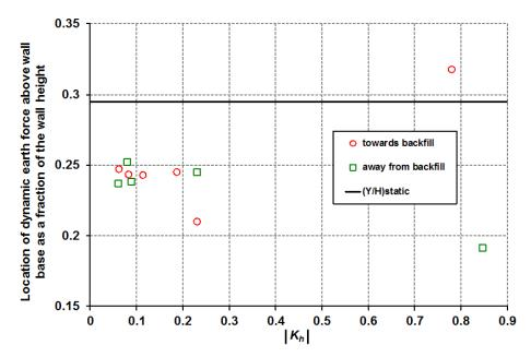
Figure 5. Point of application of total active dynamic force on sheet pile wall
