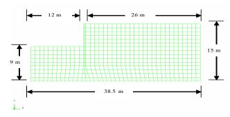
Figure 3. Annotated DIANA model of the wall-soil system
