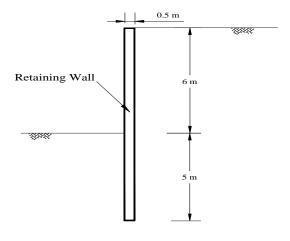
Figure 2: Dimensions of the sheet pile retaining wall
