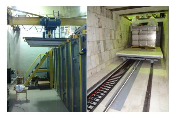
Fig. 3. General view of passive shielding: from the outside and inside. The range of detector dislocation is 6 - 12 m from the reactor core center.
