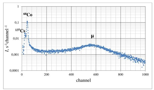
Fig. 4. Background spectrum with NaJ detector in a neutron laboratory beyond passive shielding.
