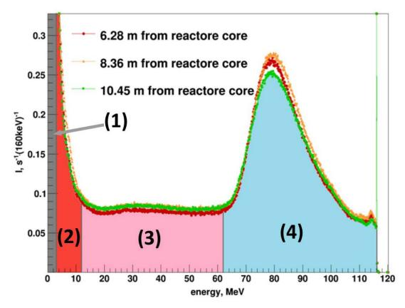
Fig. 13. Detector energy spectrum at different distances from reactor core and conventional division of spectrum into zones: 1 - radioactive contamination background, 2 - neutrons, 3 - cosmic radiation soft component, 4 -muons.
