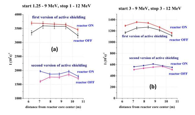
Fig. 22. a) measuring results on count rate of correlated events for start signals within the energy range of 1.25 - 9 MeV and stop signals 1 - 12 MeV at the reactor on and off, as well as for two versions of the active shielding, b) results of the same measurements for start signals within the energy range of 3 - 9 MeV and for stop signals 3 - 12 MeV.
