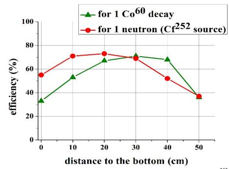
Fig. 11. Registration efficiency of neutrons and gamma-quanta from sources (<sup>252</sup>Cf and <sup>60</sup>Co correspondingly) depending on their location.
