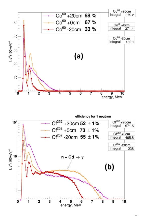
Fig. 10. Calibration of a neutrino detector model with gamma radiation source ( $^{60}$ Co) and neutron source ( $^{252}$ Cf): a) energy spectrum of  $^{60}$ Co, b) energy spectrum of  $^{252}$ Cf.
