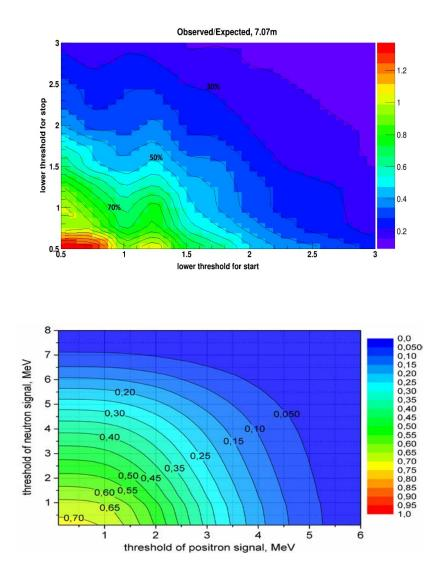
Fig. 21. a) Experimental efficiency on registration of antineutrino events depending on lower thresholds of registration of start and stop signals, b) registration efficiency of antineutrino events from Monte-Carlo calculations depending on lower registration thresholds of start and stop signals.
