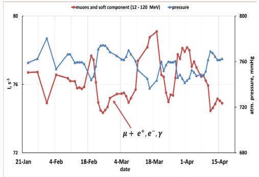
Fig. 16. Barometric effect of cosmic rays: the left axis shows summary detector count rate in the area 3 and 4, the right axis shows atmospheric pressure, horizontal axis gives the measurement time since 23d of January to 15th April 2014.
