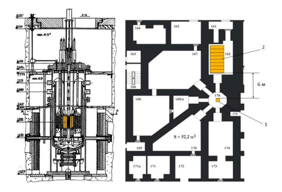
Fig. 1. Detector location at reactor SM-3: 1 – reactor core, 2 – antineutrino detector.
