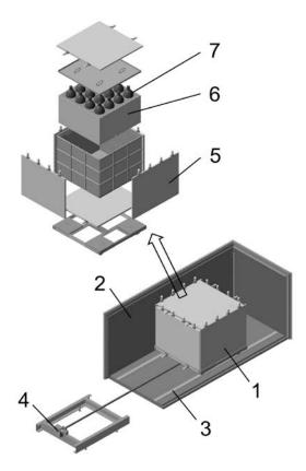
Fig. 2. Detector layout: 1 –detector of reactor antineutrino, 2 – passive shielding made of lead (6 cm) and borated polyethylene (16 cm), 3 – rails, 4 – device for detector displacement, 5 – plates of active shielding , 6 –liquid scintillator , 7 –PMT.
