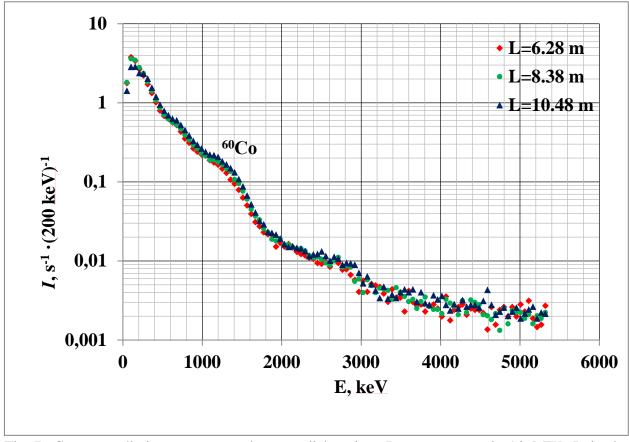
Fig. 7. Gamma-radiation spectra at detector dislocation. Reactor power is 90 MW. L is the distance from the reactor core center: -6.28 m, -8.38 m, -10.48 m.
