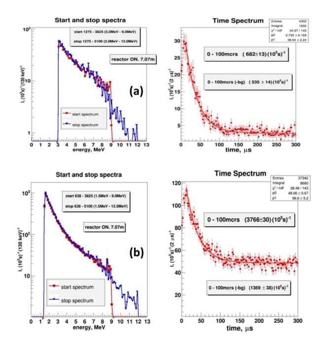
Fig. 20. Energy spectra of direct and delayed signals and time spectra: a) threshold of start and stop signals 3 - 9 MeV and 3 - 12 MeV respectively, b) 1.5 - 9 MeV and 1.5 - 12 MeV.
