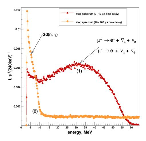
Fig. 19. Energy spectra of time delay signals in the range of  $0 - 10 \,\mu s$  (1) and  $10 - 100 \,\mu s$  (2).
