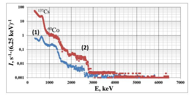
Fig. 5. Spectra of background gamma-radiation at the lead shielding (1) and without it (2), recorded with the detector NaJ (60x400 mm). Reactor power is 90 MW.
