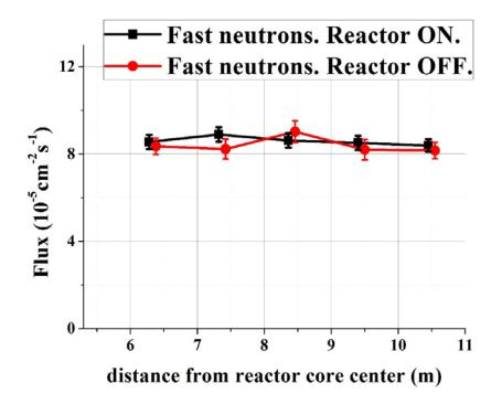
Fig. 9. Fast neutron background at different distances from the reactor core center measured with the detector of fast neutrons inside the passive shielding. The fast neutron detector was set on the cover of the neutrino detector and was dislocated together with it.
