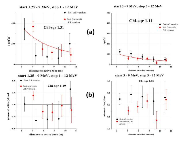
Fig. 23. a) On the left - dependence of count rate difference of correlated events (reactor on – reactor off) on distance from the reactor core center within the range of 1.25 - 9 MeV and for stop signals 1 - 12 MeV, on the right – the same for the energy range of 3 - 9 MeV and 3 - 12 MeV; b) – treatment of the same data on deviation from the law  $1/R^2$ .
