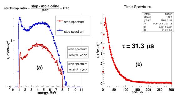
Fig. 12. a) Energy spectra of start and stop signals in Cf source experiment, b) time spectrum of neutron registration, neutron thermalization process to thermal rate is 5 -7  $\mu$ s, while thermal neutron life time in the scintillator with Gd is 31.3  $\mu$ s.
