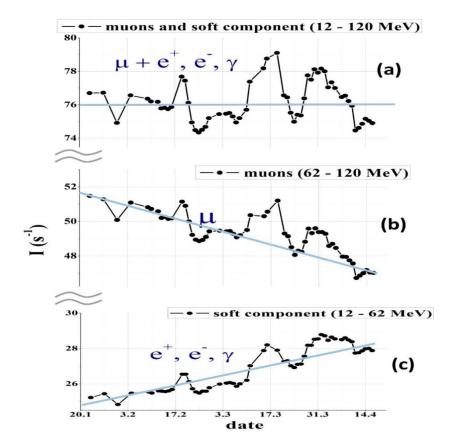
Fig. 17. Barometric and temperature effects of cosmic rays; a) summary detector count rate in the area 3 and 4, b) detector count rate in the area 4, c) detector count rate in the area 3. Along the horizontal axis is the measurement time since 23d of January till 15<sup>th</sup> of April 2014.
