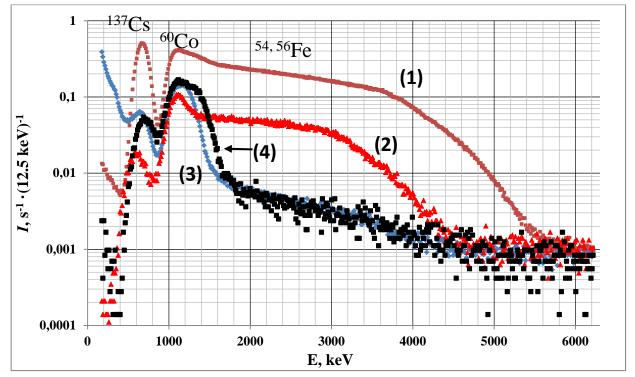
Fig. 6. Distribution of gamma-radiation intensity on the roof of the passive shielding at the distances of 1 m (curve 1) and 7 m (curve 2) from the reactor wall, as well as inside a cabin at the distance of 0.5 m (curve 3) from the reactor wall. Reactor power P=90 MW. Spectrum 4 is recorded when the reactor is off, at the distance of 9 m from the reactor wall, on the building floor.
