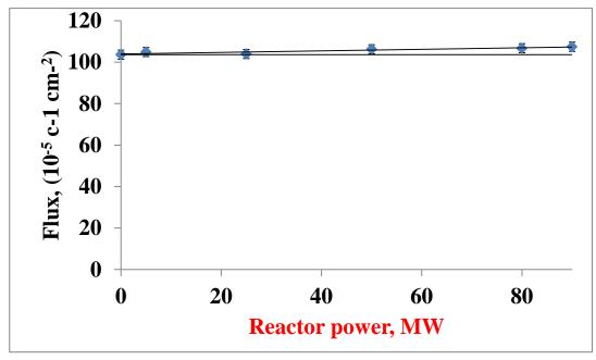
Fig. 8. Flux of a fast neutron detector at output power reactor 90MW. The counter is located on the cabin roof at the reactor wall.
