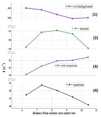
Fig. 14. Dependence of the detector count rate in different ranges of energy spectrum of a neutrino detector model (enlarged scale with discontinuities) 1 - radiation contamination background, 2 - neutrons, 3 - cosmic radiation soft component, 4 - muons.
