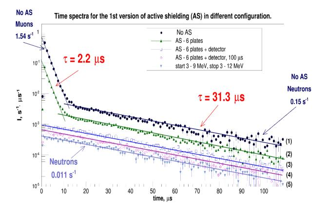
Fig. 18. Time spectra at different configurations of the active shielding: 1 - no active shielding, 2 – plates of the active shielding are on, 3 – the same + ban from the detector at signals higher than 12 MeV, 4 – the same + ban on 100  $\mu$ s after the detector signal, at energy higher than 12 MeV, or after the signal in the active shielding, 5 – the same + limit on start and stop signals in ranges 3 – 9 MeV and 3 – 12 MeV respectively.
