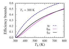
**Figure 2.** Efficiency bounds as a function of the temperature of the hot source  $T_h$  for fixed  $T_e = 300$  K. The near-field efficiency  $\overline{\eta}_{nf}$  is plotted for hBN, and for comparison also the Carnot efficiency  $\eta_c$  is plotted.
