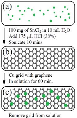
Remove grid from solution Wash with deionized water Dry at 70°C for 12 hours
