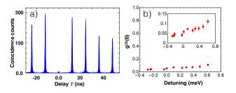
FIG. 2: a) Autocorrelation histogram on QD–cavity resonance, from which we extract  $g^{(2)}(0) = (0.058 \pm 0.006)$ . b) Autocorrelation function as a function of QD–cavity detuning (the inset shows a zoom-in of the y-axis).
