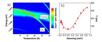
FIG. 1: a) Temperature dependent intensity map of the QD-cavity system. The QD reaches spectral resonance with the cavity mode at  $T=17.5~\mathrm{K}$ . b) QD lifetime as a function of QD-cavity detuning. The fit is a Lorentzian profile where the linewidth is fixed to the cavity linewidth. A Purcell enhancement of  $F_P=7.8\pm2.3$  is extracted.
