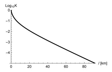
Figure 1. The secret key fraction K as a function of the distance between Alice and Bob assuming a loss coefficient of 0.2 dB/km and the optimal  $\gamma$  for the specified distance. This plot gives the raw fraction; it does not include finite detection efficiencies, dark counts, thermal noise, or the relative sampling frequency of the  $\{A_0, B_1\}$  measurement.
