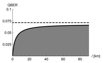
Figure 2. Plot of the critical QBER  $Q_{\rm crit.}$  as a function of distance, see text for details. The biphoton approach is superior in the gray region, corresponding to  $Q < Q_{\rm crit.}$ . The phase-entangled coherent state approach is superior in the white region, corresponding to  $Q > Q_{\rm crit.}$ . The discrete variable diQKD approach using biphotons cannot be used when the QBER exceeds the dashed black line.
